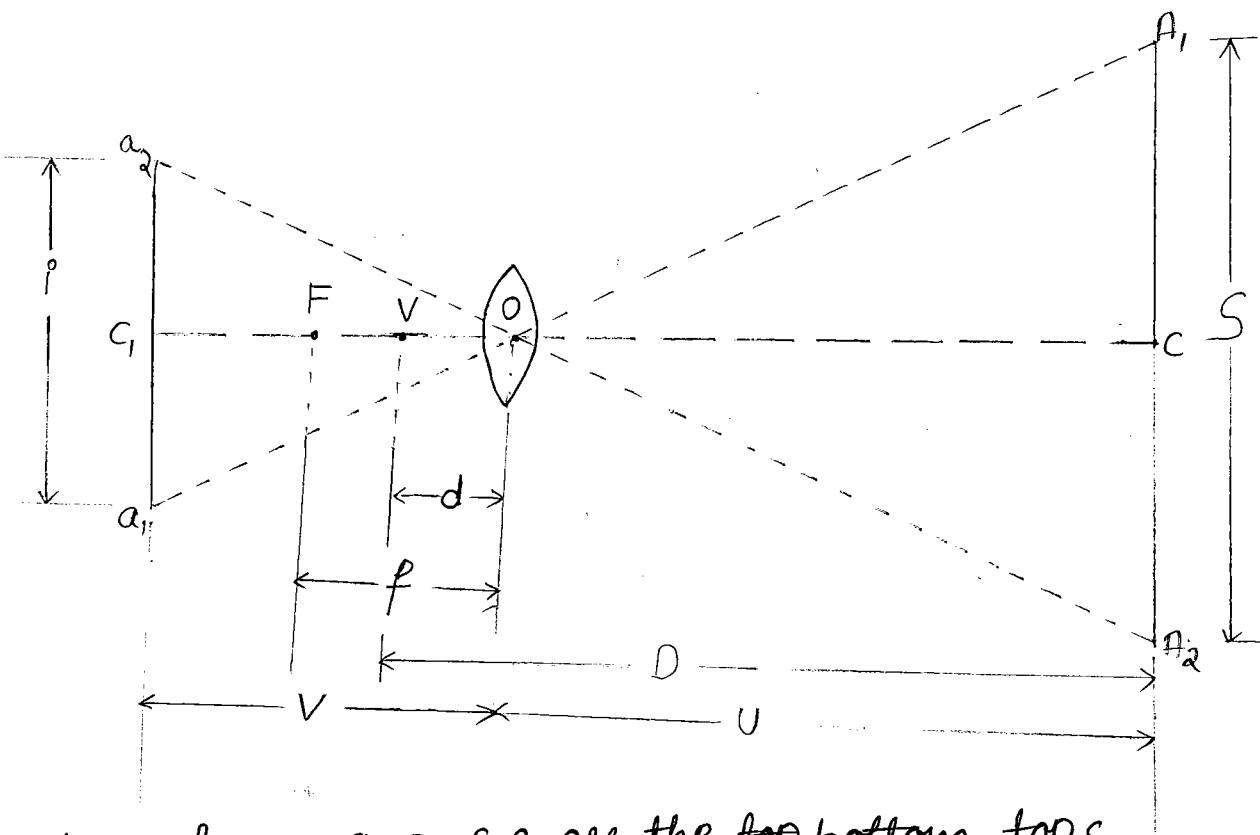
In the above figure,  $a_1, a_2$  &  $c$ , are the ~~top~~ bottom, top & central hairs of diaphragm.  $A_1, A_2, C$  are readings on staff cut by three hairs.
